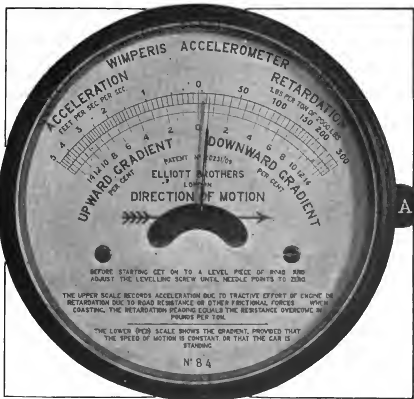
The dial of the accelerometer and directions for its use and adjustment as printed thereon
